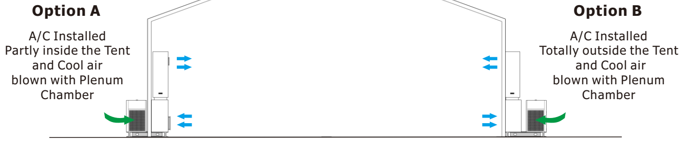
Demonstration of A/C Installed Inside and Outside the Tent
