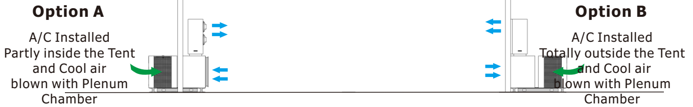
Demonstration of A/C Installed Inside and Outside the Tent
